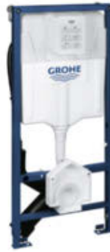
39 112 001 Rapid SL for shower WC flushing cistern GD 2 with small maintenance access 1.13 m installation height, pipe for GROHE Sensia water inlet, socket for mains supply
