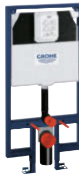
38 994 000 Rapid SL for WC for small, narrow bathrooms flushing cistern 80 mm with small maintenance access 1.13 m installation height element width 0.62 m
