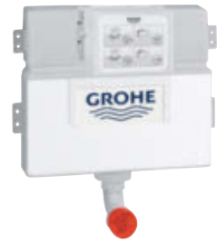
38 422 000 Flushing cistern for WC 6 l / 3 l Dual Flush 0.82 m finished installation height front/top actuation water supply from left/right or back Insulated against condensation without wall plate/actuation & flush pipe
