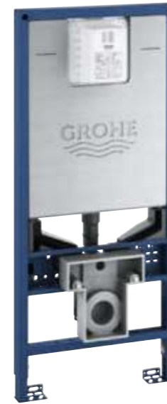
39 597 000 Rapid SLX WC 3-6 | 1.13 m, without outlet pipe Rapid SLX Element for WC, 1.13 m installation height with flushing cistern GD2, with electric socket, including flow manager, easy access and fully insulated against condensation. Without outlet pipe.
