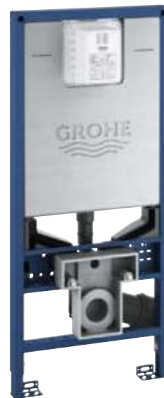
39 596 000 Rapid SLX WC 3-6 | 1.13 m, Standard Rapid SLX Element for WC, 1.13 m installation height with flushing cistern GD2, with electric socket, including flow manager, easy access and fully insulated against condensation.
