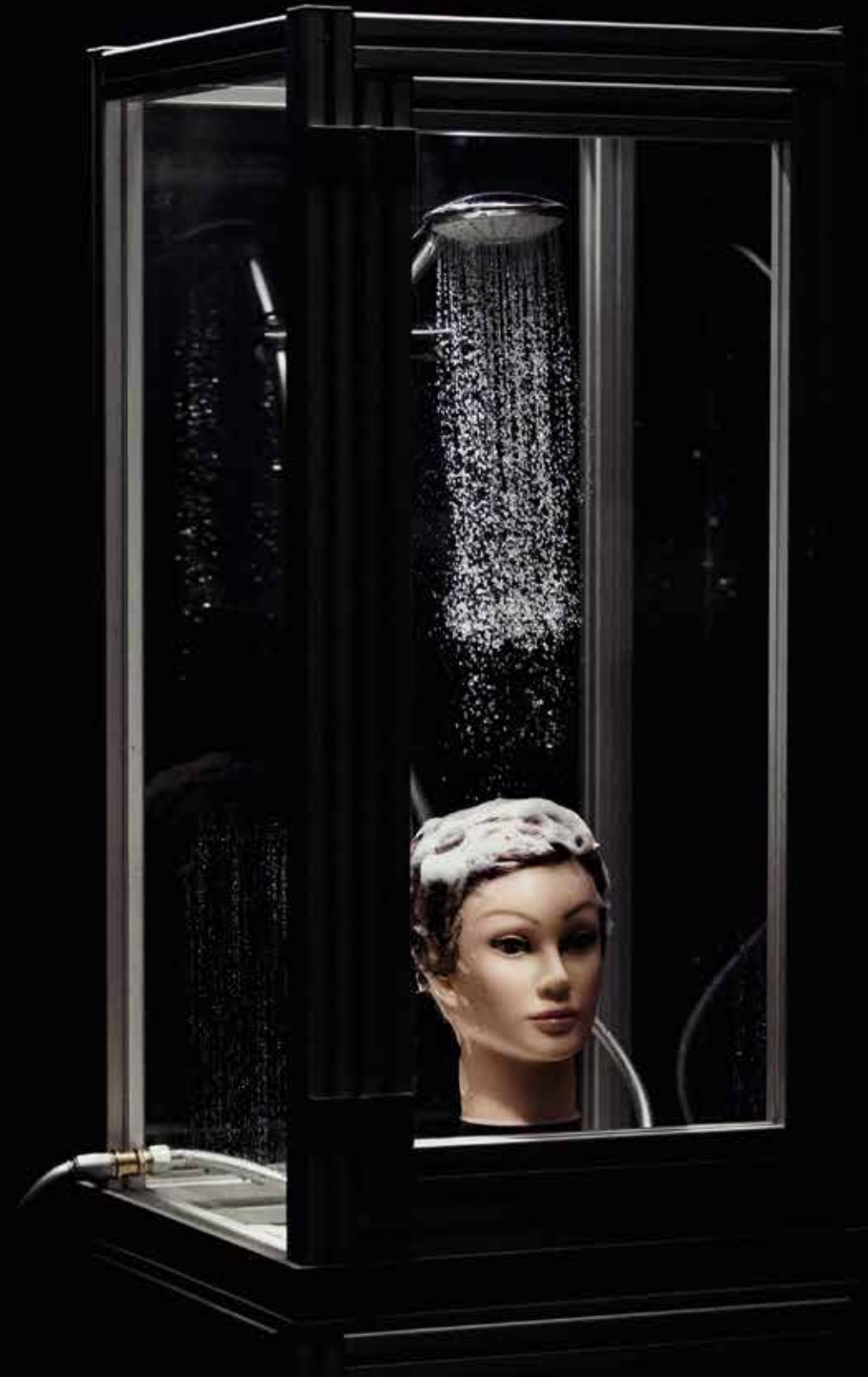
Bensing's shower lab examines shower head spray patterns, analyzing how they can be optimized to save water and increase efficiency.
