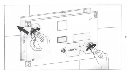
Fix the control plate base to the cistern with two long plastic screws as picture F.
