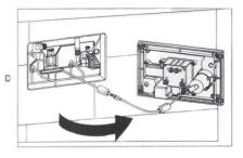
Connect the DC connector with magnetic ring of the transformer to the DC base at the back of the control plate as picture D.
