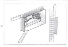
Cut the protecting frame to the level of the wall with a knife as picture B.
