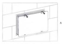
After completing the cistern installation and wall treatment, remove the protecting cover as picture A.
