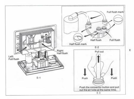
Cross-connect the two air tubes to the air holes at the control plate base as picture E-1.
