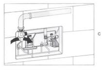
Clockwise rotate the valve handle in the cistern to open the valve as picture C.
