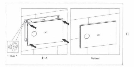
Installation: Press the four corners of the glass plate after alignment to lock the 4 snap joints.
