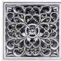
0303-71-79CP Floor Drain Brass Size 100*100 mm Height 61 mm Seal Type Self Seal Brass Flow Rate ≥15L/Min Outlet OD 40 mm Drain Core 0303-A1-7900
