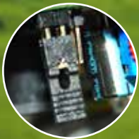
ON / OFF jumper for heating element Option to turn on/off the heating element
