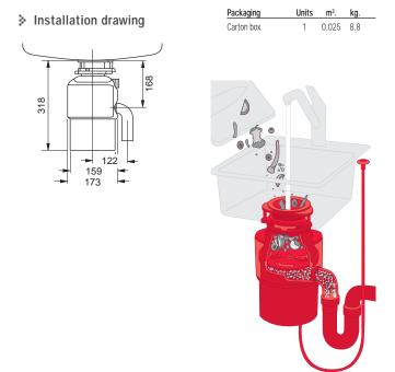
Teka food waste disposer can be installed on sinks with 3 1/2" basket waste. This waste device is easy to install, easy to operate, reliable, and produces innumerable benefits for the user and for the environment. Accumulated garbage can attract insects, and produce unsanitary conditions around your home. Due to the Teka food waste disposer, food waste (chicken bones, fruit rinds,...) is milled into fine particles that are eliminated through the sewage system.
