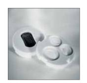
» All Teka cartridges use sintered ceramic discs of high resistance. These discs all have porous surfaces which retain the grease longer helping to achieve smoother, gentler movements and therefore prolonging the life of the taps. The operating gear is insulated from water giving therefore continuous lubrication.
